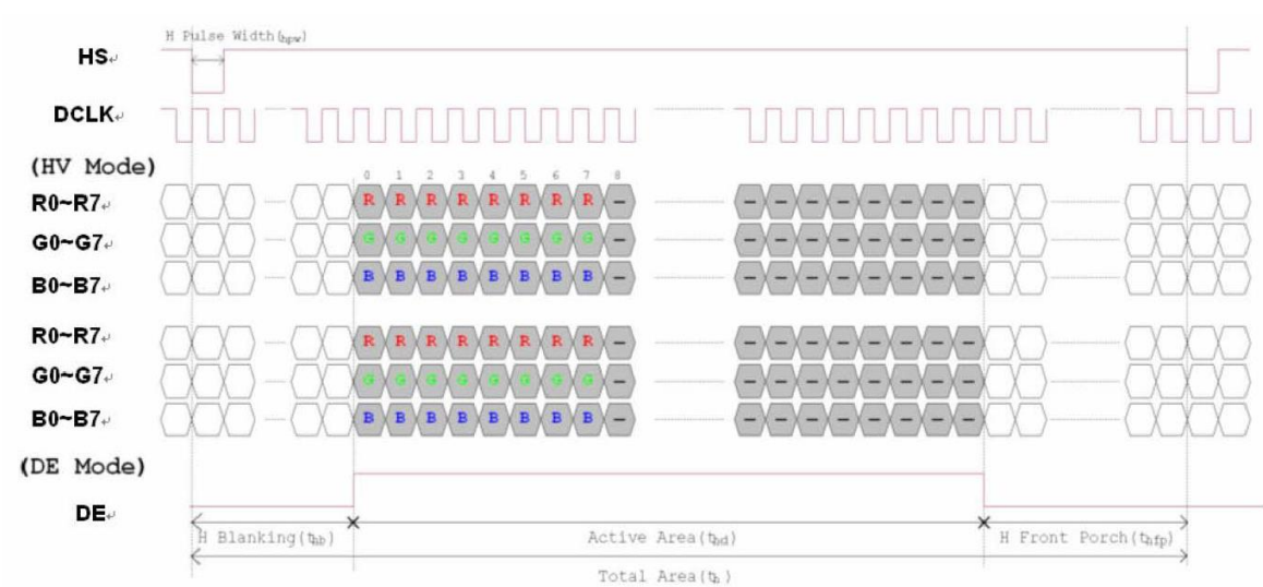
Figure 1. Horizon input timing diagram
